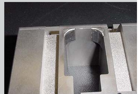
Changing the radius on the matrix of a punching tool of 1.2379 (Photo: L&A Lasertechnik, Radebeul)
