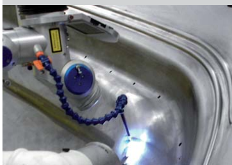
Repair welding (Photo: PML Lasertechnik, Nohra)
